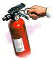
P ull the extinguisher's safety pin
